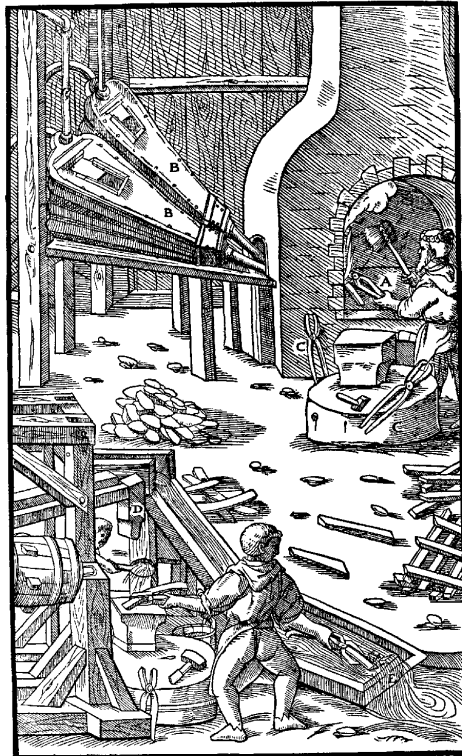
A—FORGE. B—BELLOWS. C—TONGS. D—HAMMER. E—COLD STREAM.
